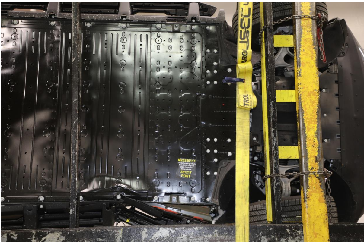
305-35 Post-Impact View of Battery Component Intrusion
