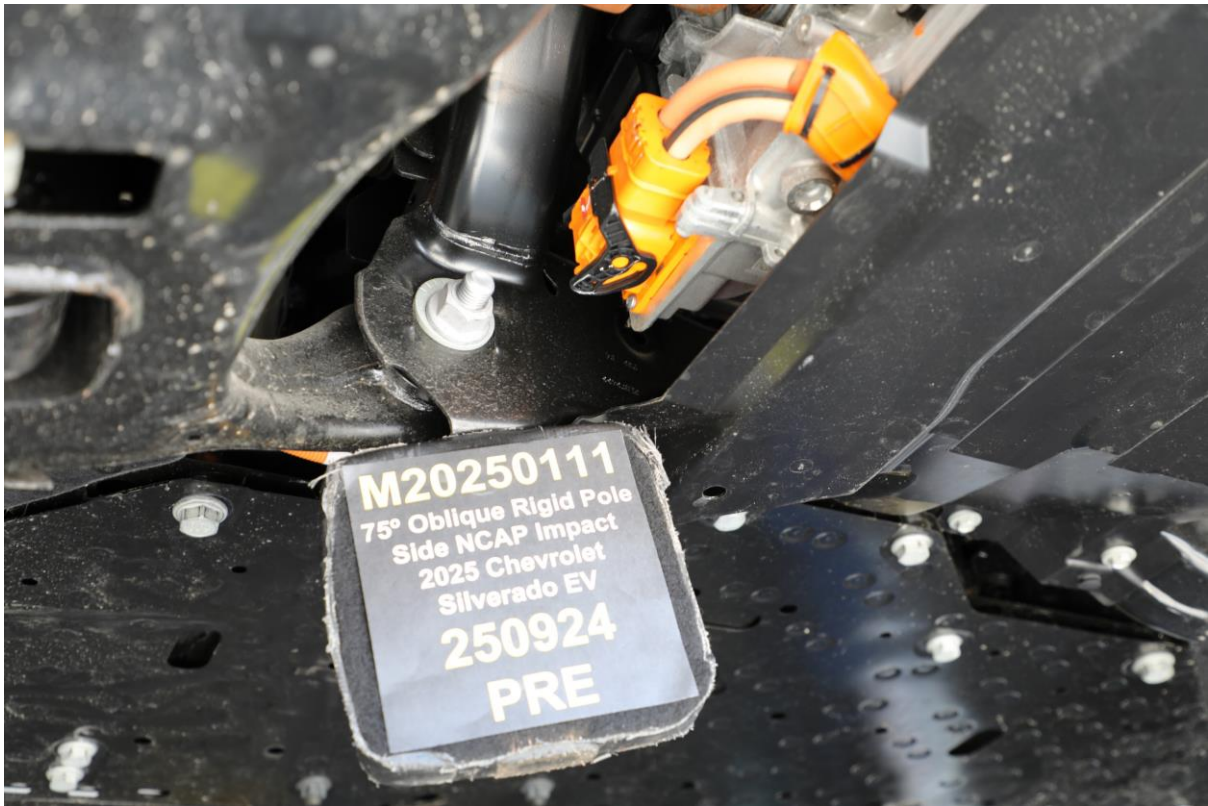
305-18 Pre-Impact View of High Voltage Interconnect(s)
