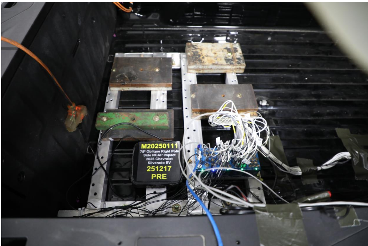
No. 063 Pre-Test Ballast View
