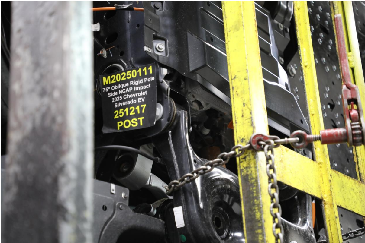
305-10 Post-Impact Front View of Propulsion Battery
